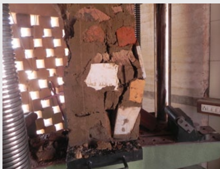
Debris Wall Testing
