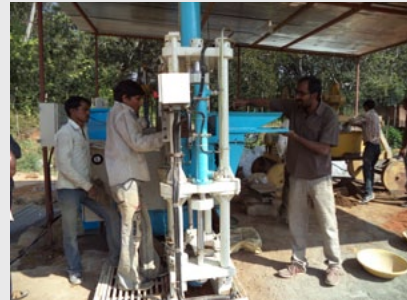
The hydraulic press designed with Gram Vidya
