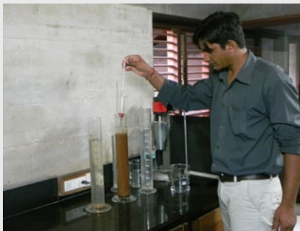
Hydrometer test performed in the Hunnarshala lab
