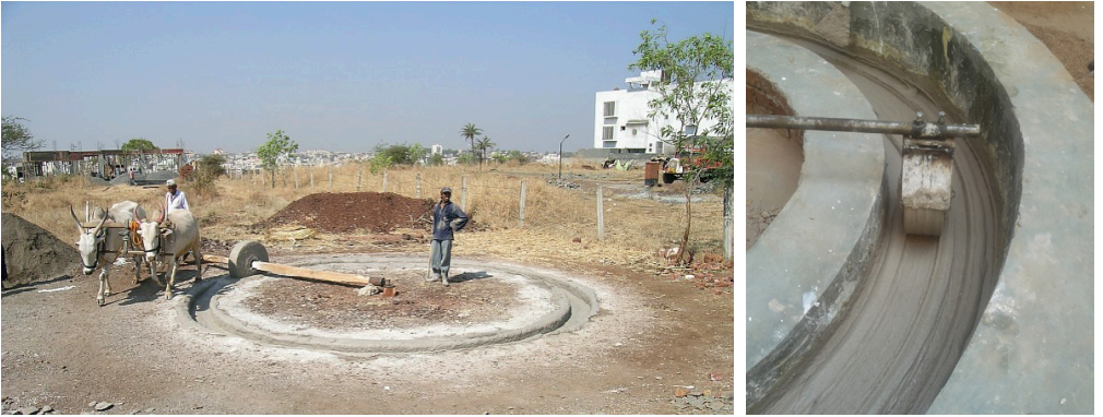
Figure 18. Bullock driven traditional mill for lime hydration
