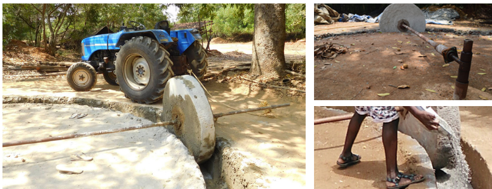
Figure 22. Lime chakki, wheel fixing at centre, pouring of material in track at Sacred Groves, Auroville
