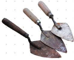
Figure 29. Mason's trowel (Chunaidu)
