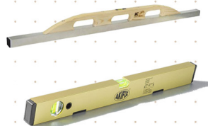
Figure 40. Straight edge; Spirit Level
