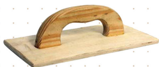
Figure 45. Steel floats (Malo) and wooden floats (Randho, randhli)
