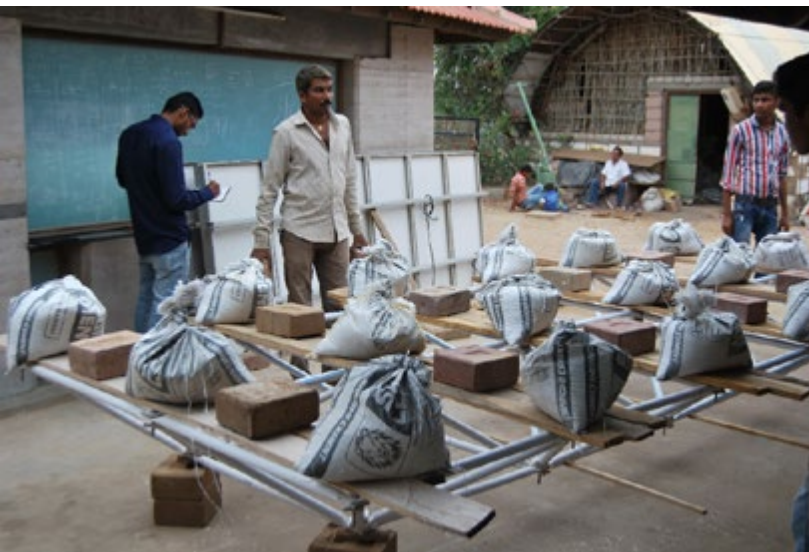
Load testing of spaceframe made out of PVC pipes
